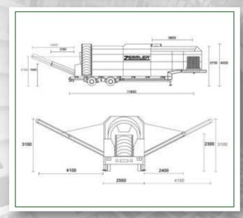
up to 180 m<sup>3</sup>/h **Troughput Trommel length** 6.700 mm
