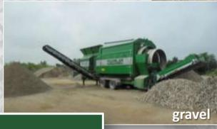
Our **MULTI SCREEN®** screens can be used in different fields of application. Due to the double trommel technology it is possible to screen various material into 3 fractions in just one working stage. The exchangeable wire screens allow the optimum adaptation to any screening requirements.
