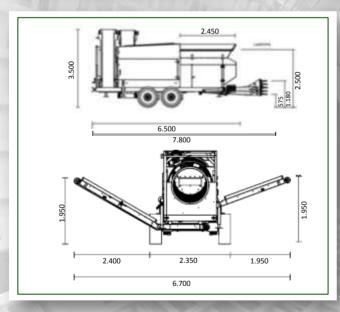
**Troughput** up to 60 m<sup>3</sup>/h **Trommel length** 3.000 / 3.900 mm Trommel-1.300 mm Diameter Mesh size 2 up to 80 mm Screening ca. 18,1 m<sup>2</sup> surface total Weight ca. 5.500 kg electric, Drive optional fuel aggregate Hitch Drawbar eye Ø 40 or 50 mm
