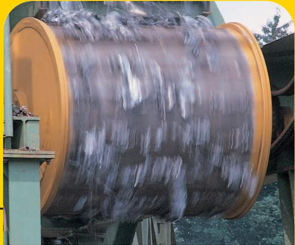
Applications such as pre-separation of ferrous before Eddy-Current separators and recovery of slightly magnetic material found in crushed batteries or electronic scrap take advantage of
