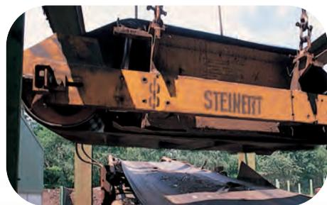
the treatment of slags and pyrolysis coke from thermal refuse treatment. **STEINERT** suspension magnets, mostly permanent magnet models, can be used to process iron-free demolition scrap into a valuable building material. Smaller iron particles, which are not captured by the drum magnet immediately behind the shredder, are extracted from the heavy shredder fraction. Bottle caps and screw tops are removed from collected glass for recycling before it is remelted.
