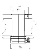
Installation example in the discharge chute of a sorting plant
